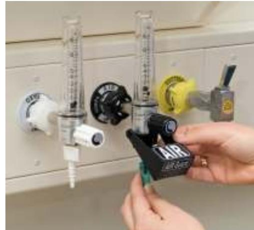
*Fig. 2: Attaching patient tube with AIR Guard*
